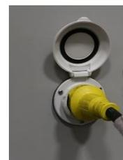
When your trailer is hooked up to external AC power, the converter system automatically charges the trailer battery(s) with the battery disconnect switch in the ON position. If the 7-way cord is hooked up and depending on your vehicle, your tow vehicle will
