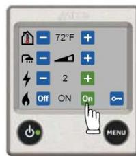
To light the Alde system on propane, press the Propane icon “On”, on the thermostat. The On icon is activated and changes color to green. As seen in the photo.
