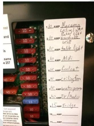
Each 12 VDC circuit in the distribution panel was designed for a maximum of a 20-amp automotive style fuse. Should one need to be replaced, be sure to replace it with the same type and Amp rating as originally supplied by **nüCamp RV**.
